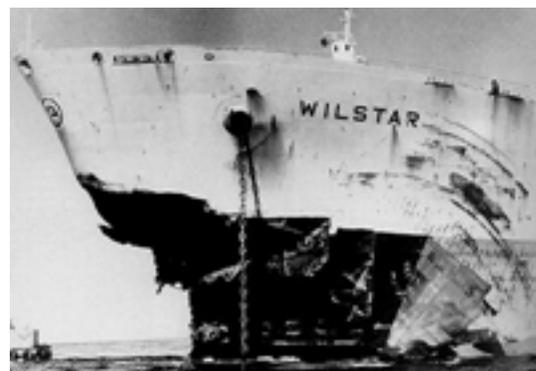
*Bow damage caused by a giant wave*
